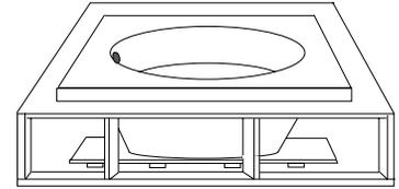
**To insure proper drainage**, use a 4 ft. level to level the top of bathtub in both directions, do this before mortar is dry.
